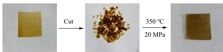
Fig. 11 Reprocessing of H-TPI films by hot-press method using H-TPI-2 film as an example.
