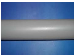
Fig. 1 The photograph of the PE pipe obtained via rotation extrusion
