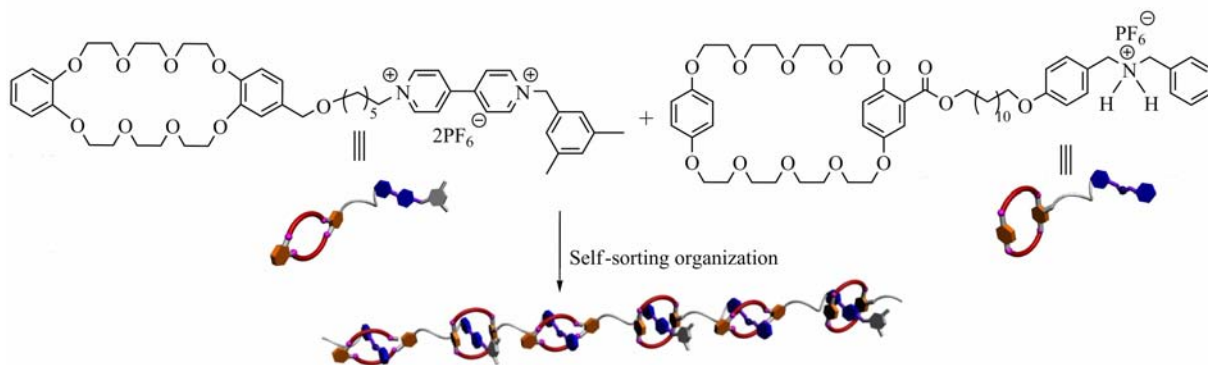
Fig. 2 Self-sorting organization of two heteroditopic monomers to supramolecular alternating copolymers [26] (Copyright 2008 American Chemical Society)
