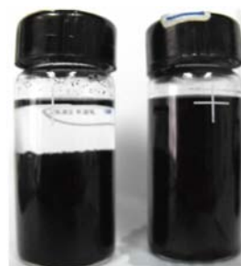
Fig. 6 Pictures of MWCNTs in DCB for 7 days, MWCNTs (left) and β-NA-MWCNTs (right)
