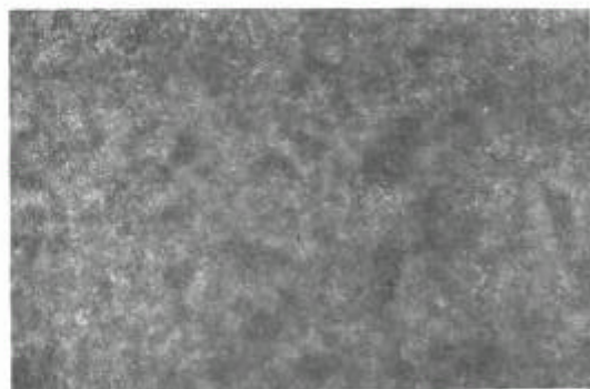
Fig. 3 Optical photograph texture of polymer P-II annealed for 5 h at 190°C
